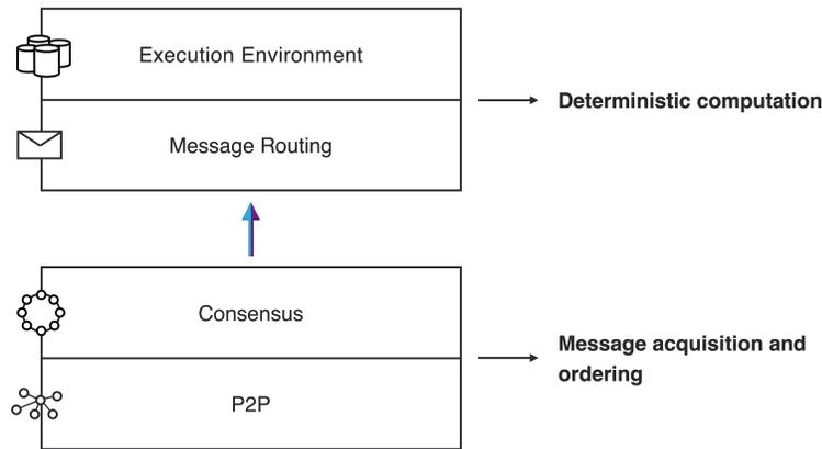
Figure 1: The layers of the Internet Computer Protocol
